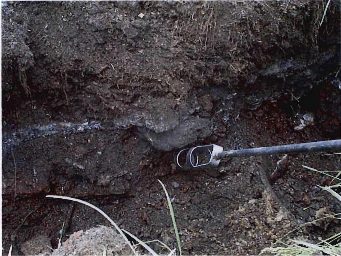
Photo #2: Fire Training Pit, Exploratory Trench FTA-TR2, 24 May 2001 "Landfill Trench / Secondary Burn Pit" Area Ash Layer Visible in Trench Wall
