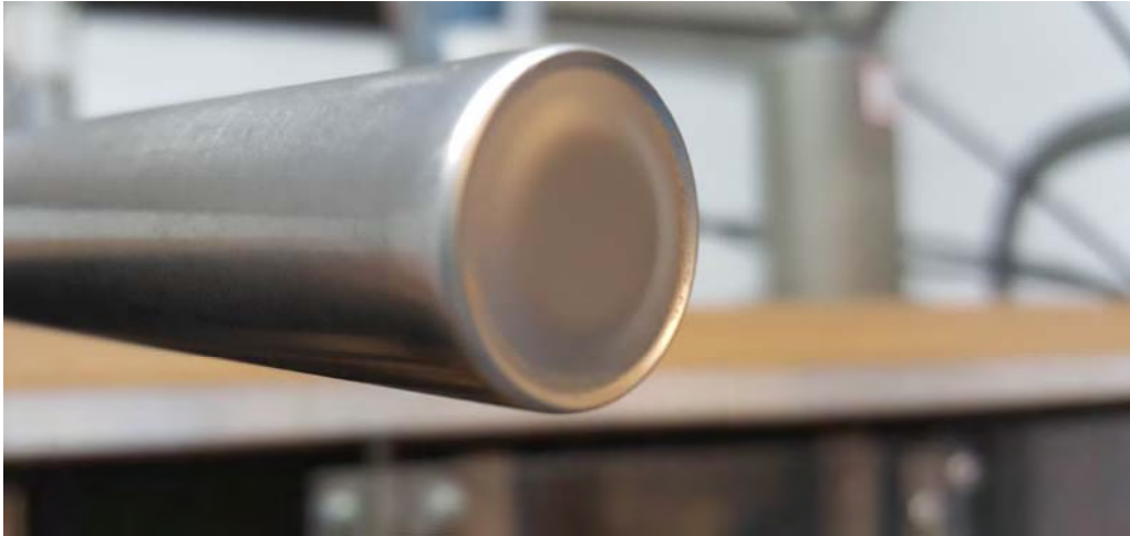
Condition: poor; heavy pitting, replace horn.
