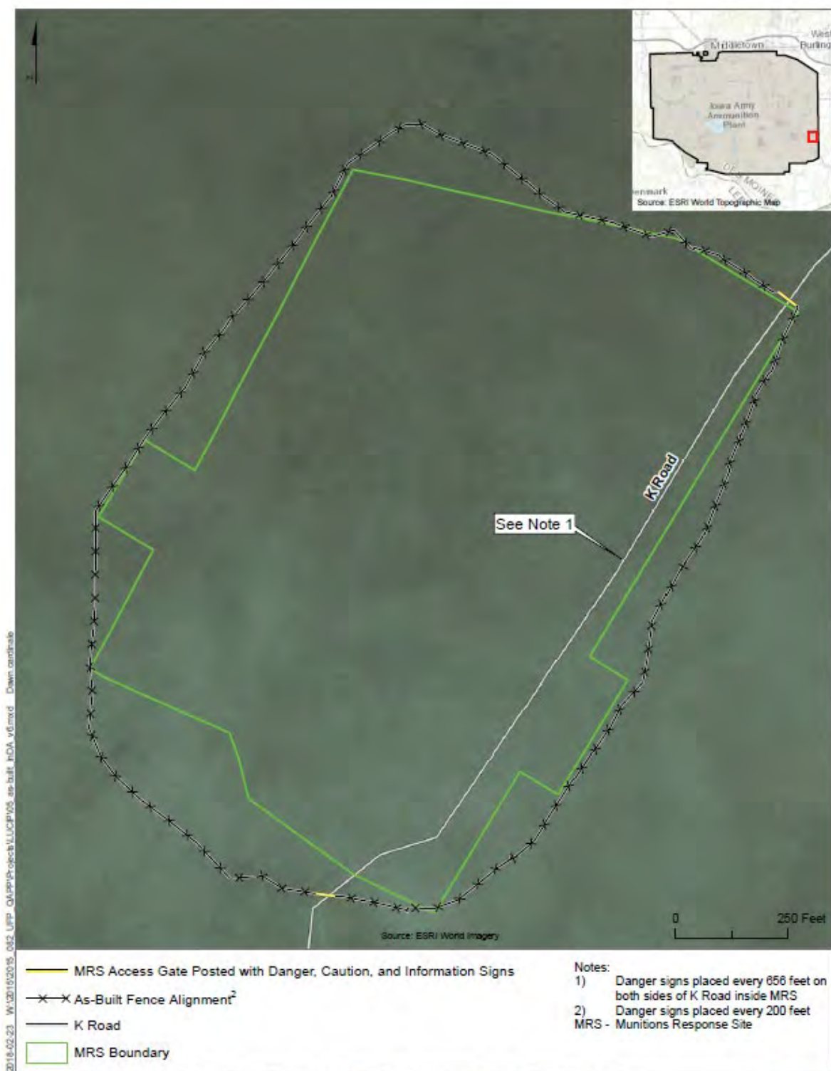
Figure 5. As-Built Fencing Layout for the Incendiary Disposal Area Annual Land Use Control Implementation Report, Operable Unit 5 Munitions Response Sites Iowa Army Ammunition Plant, Middletown, Iowa
