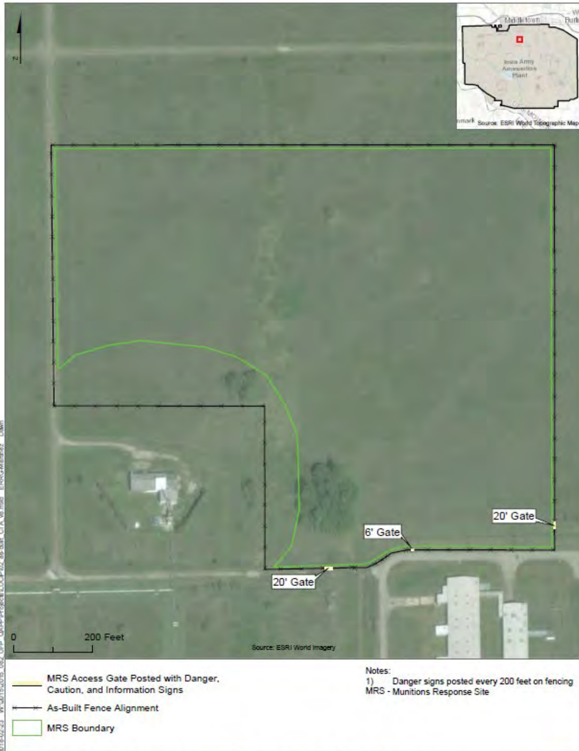
Figure 2. As-Built Fencing Layout for the Central Test Area Annual Land Use Control Implementation Report, Operable Unit 5 Munitions Response Sites Iowa Army Ammunition Plant, Middletown, Iowa
